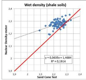
Fig. 4 Nuclear density-meter vs sand cone tests results for the wet density in shale soils.
