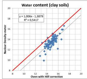
Fig. 2 Nuclear density-meter vs sand cone tests results for the water content in clay soils.
