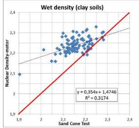
Fig. 1 Nuclear density-meter vs sand cone tests results for the wet density in clay soils.
