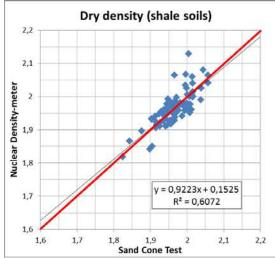
Fig. 6 Nuclear density-meter vs sand cone tests results for the dry density in shale soils.
